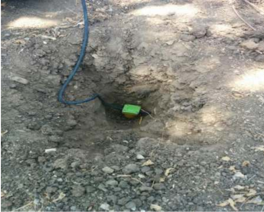
Placing the sensor in the pit
